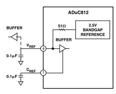
Figure 9. Decoupling  $V_{REF}$  and  $C_{REF}$
